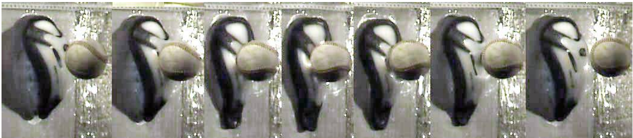
A Brand - 2 cup being struck in the center at 60 MPH. Note, in the 4 th photo of the sequence, how the cup appears to flatten completely.
