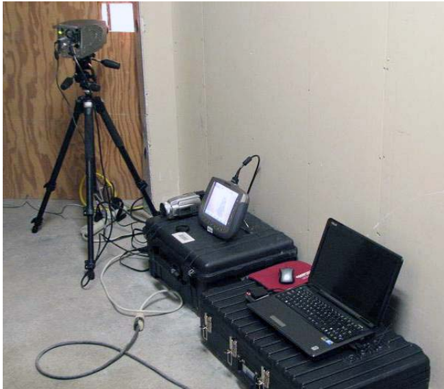
The camera setup. Note the small, Lexan-covered window through which the camera photographed the baseball hitting tested cups.
